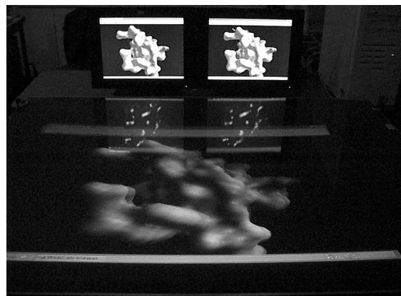
Figure 4. Sterographic table showing a stereo image of protein relaxin. LCD panels (at top) display left and right images.
