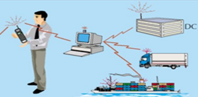
RFID reads item in inventory at a store or DC plus items in transit so company knows up-to-date inventory status and can synchronize supply chain
