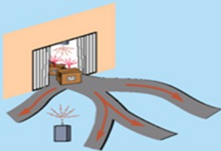
RFID directs packages through a conveyor system in distribution center
