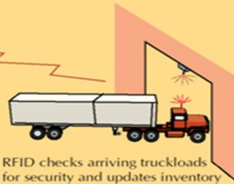
RFID reads item in inventory at a store or DC plus items in transit so company knows up-to-date inventory status and can synchronize supply chain
