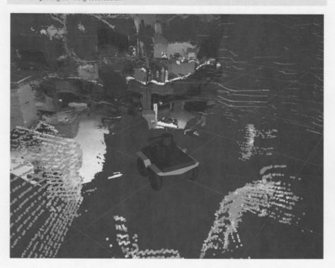
You can rotate the model using your cursor, and zoom in or out by scrolling up or down. Strafe by holding down Shift and dragging the model. The robot itself may be driven directly from rviz by changing to interact mode. In this mode, arrows appear around the model. Drag the arrows to make the robot move.
