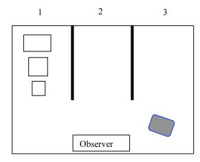
The robot (gray) must move the three boxes from the leftmost column to the rightmost. It can push or lift one box at a time. A box can never be in front of a smaller box, as seen from the observer. The larger a box is, the taller also. The front area must be kept clear so the robot can move; there can be no boxes left in this area.
