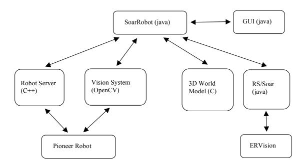
The above diagram shows the major components of ADAPT. The lower left part of the diagram shows the two components that run on the PC that is onboard the Pioneer Robot. These are the robot server software that provides the basic interface to the robot, and the bottom-up component of the Vision System, which provides basic visual data including stereo disparity (distance information), segments (color blobs), and optical flow (motion information). The
