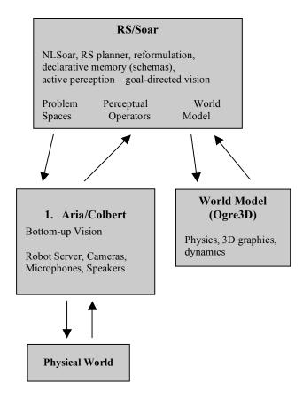
So the gaming platform provides ADAPT with a means of "understanding" the world by creating and manipulating a virtual copy of it. The gaming platform's objects are connected with Soar working memory elements, which permits Soar to reason about and talk about its model of the world.
