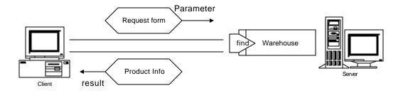
The purpose behind RMI is to make all the implementation details transparent to the programmer so that remote objects and methods work just like the local objects and methods.
