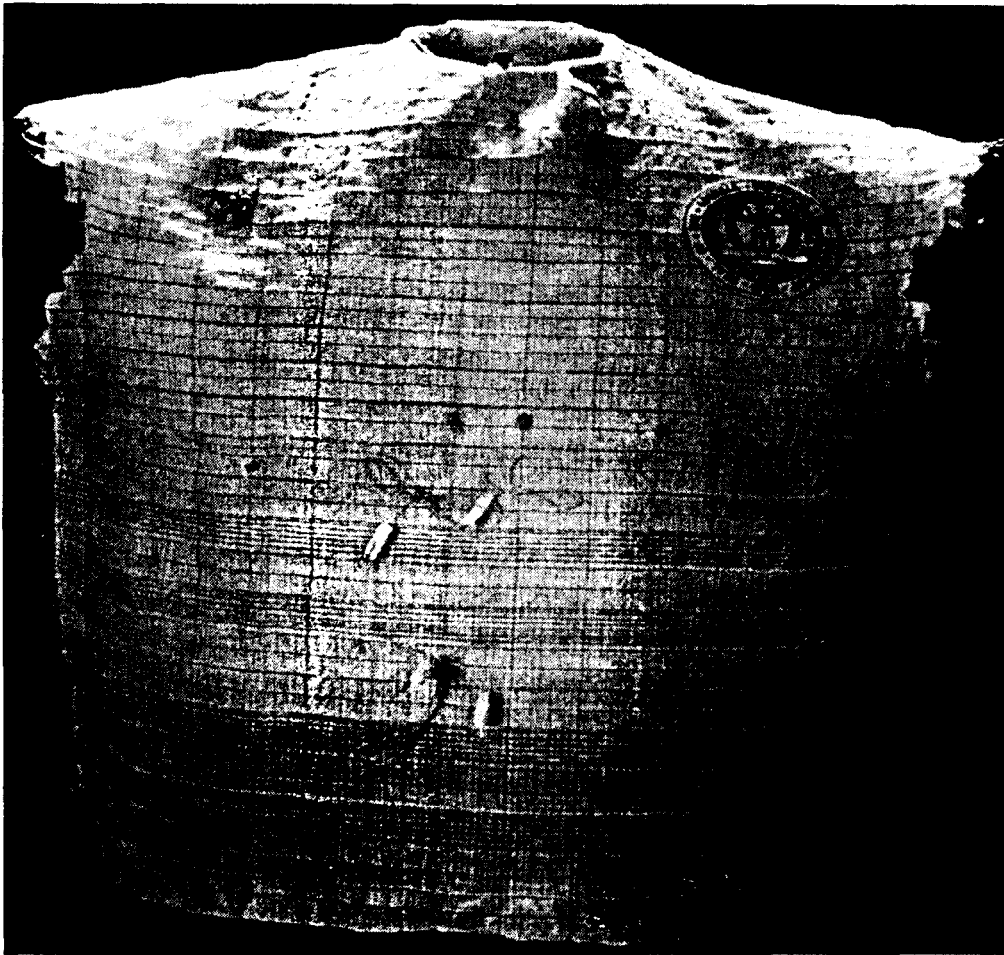
FIG. 15.4. Sensate liner developed by Lind, Jayaraman, Rajamanickam, Eisler, and McKee (I 997) at the Georgia Institute of Technology ( http://vishwa.tfe.gatech.edu/gtwm/gtwm.html ).
