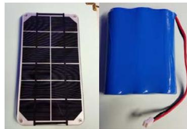
Fig. 7. Solar Panel and 3.7v Power Cell
