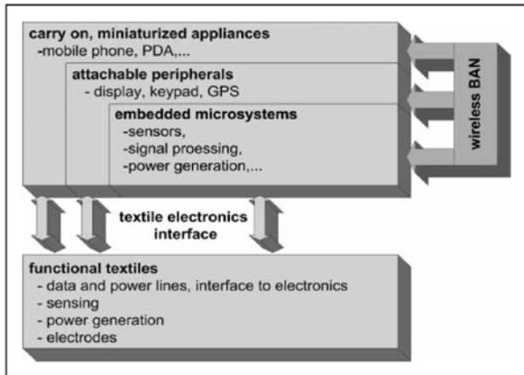
Figure 2 - Wearable Device Architecture [8]
