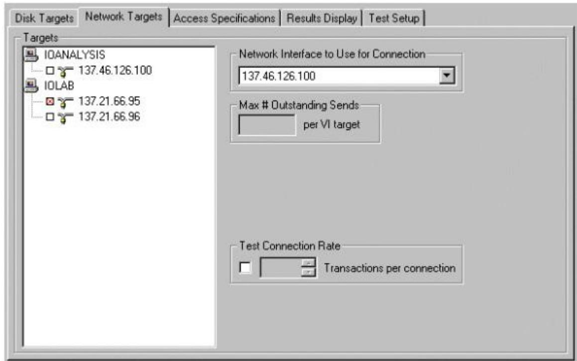
The Network Targets tab lets you see and control the network interfaces used by the network worker(s) currently selected in the [Topology](#) panel. You can control which network interface is used on each end of the connection and how frequently the network connection is opened and closed. Iometer currently supports the TCP/IP and Virtual Interface Architecture network protocols.
