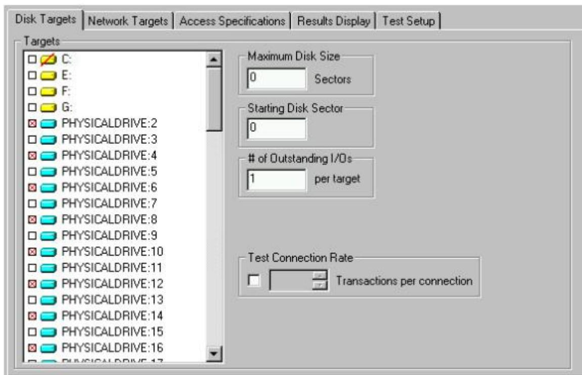
The Disk Targets tab lets you see and control the disks used by the disk worker(s) currently selected in the [Topology](#) panel. You can control which disks are used, how much of each disk is used, the maximum number of outstanding I/Os per disk for each worker, and how frequently the disks are opened and closed.
