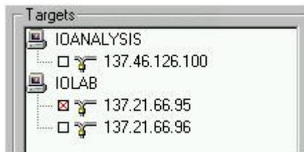
Click to select network interfaces for network server(s) (at most one per server). Control-click to deselect the currently-selected interface. A network client is automatically created on the selected manager to communicate through the selected interface on that manager.
