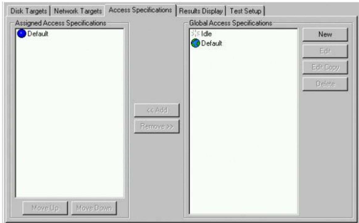
The Access Specifications tab lets you see and control the type of I/O each worker performs to its selected target(s).
