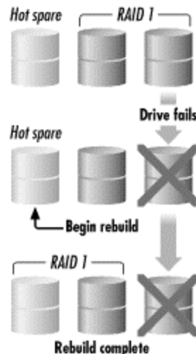
Figure 10-13. Automatic recovery of data in a redundant disk array to a hot spare
