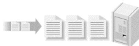
Figure 1-2. Simple model of a queuing system showing customer requests arriving at a single server
