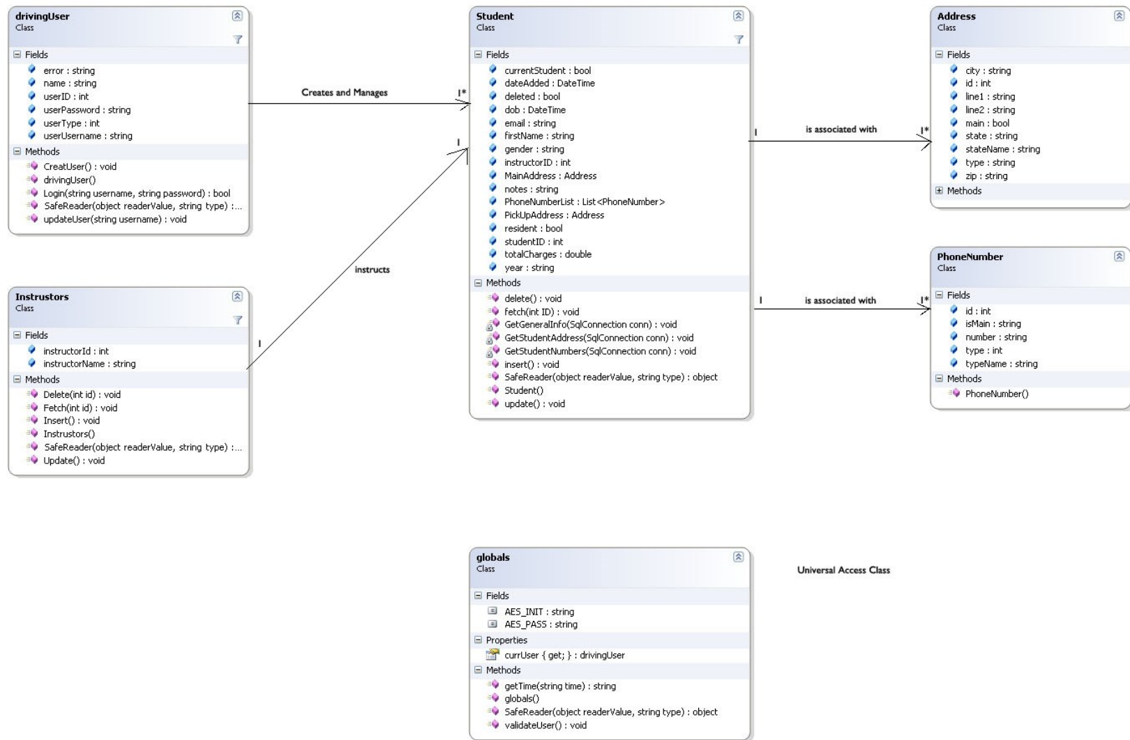
Figure 2: Domain Model diagram depicting all classes that are currently implemented in the Manhattan School of Driving system and their relationship with each other.
