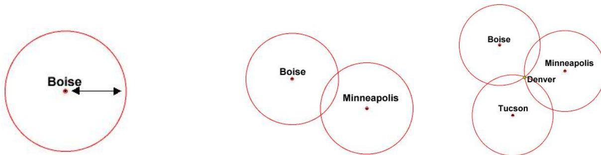
**Figure 2.** Principle of trilateration in 2-D space
