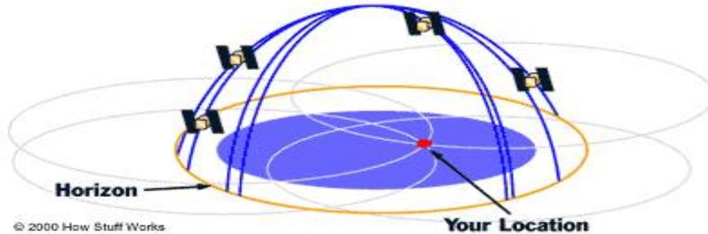
**Figure 3.** Principle of trilateration in 3-D space as used in GPS.
