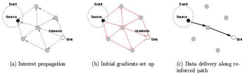
**Figure 5.** Schematic diagram for directed diffusion
