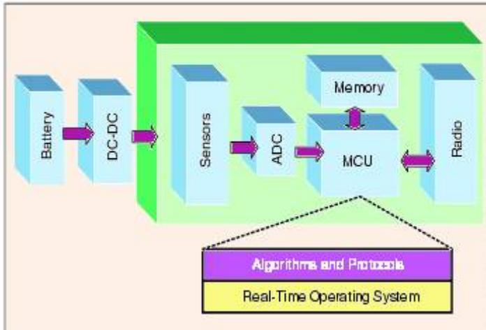
**Figure 1.** System architecture of a typical wireless sensor node
