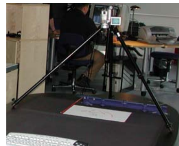
Figure 11: The first working prototype of the “Snap-scanner” allowing taking a snapshot and linking a tag to the physical material in one operation.
