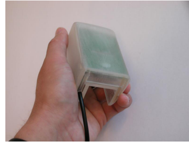
Figure 8: The small hand-held RFID tag-reader.
