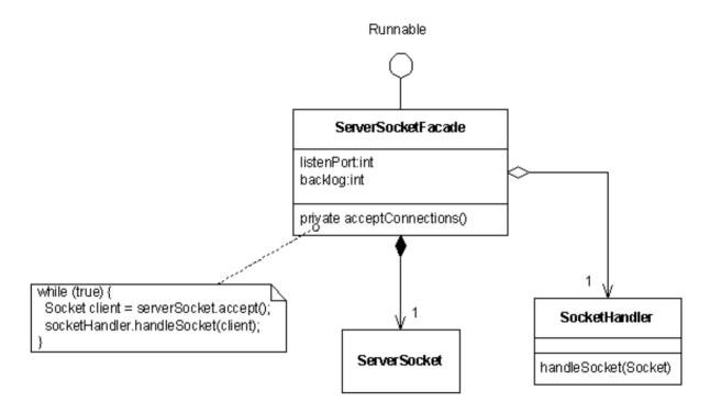
We wrapped our ServerSocket in a ServerSocketFacade, which is Runnable and owns an instance of a ServerSocket. Our applications can instantiate a ServerSocketFacade with a particular server-side port to listen to and a maximum number of client connections allowed (the default is 50). The application then runs the Facade in a new Thread to hide the ServerSocket interaction details.
