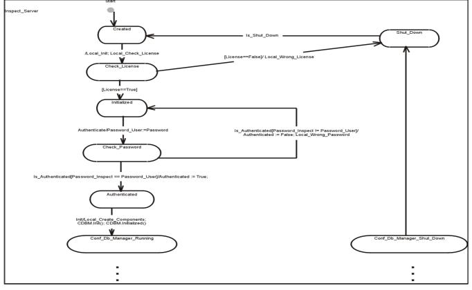
Figure 4 Fragment of the statechart of the class inspect\_server
