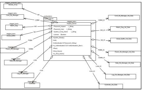
Figure 3 The structure of Inspect 2 as class diagram
