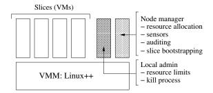
Figure 1: PlanetLab Node Architecture
