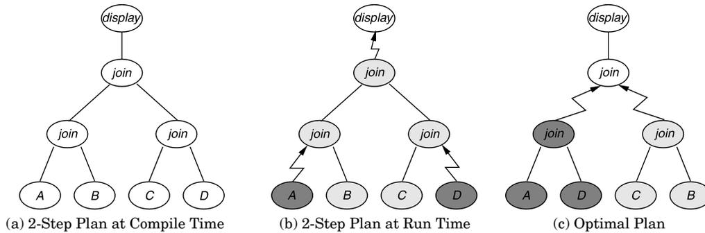
**Fig. 11.** Increased communication cost due to two-step optimization.
