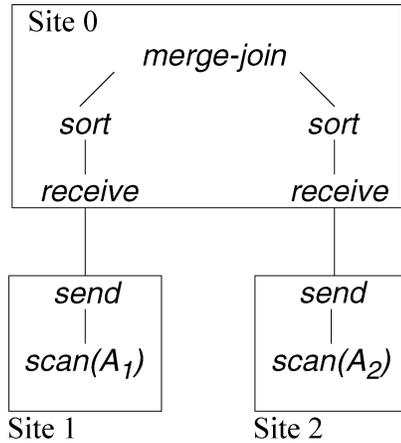
Fig. 6. Example join plan.
