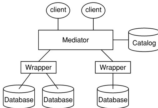
Fig. 12. Wrapper architecture of heterogeneous databases.
