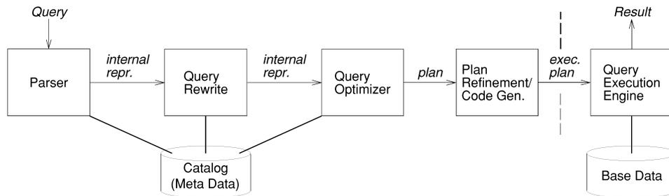
Fig. 1. Phases of query processing [Haas et al. 1989].
