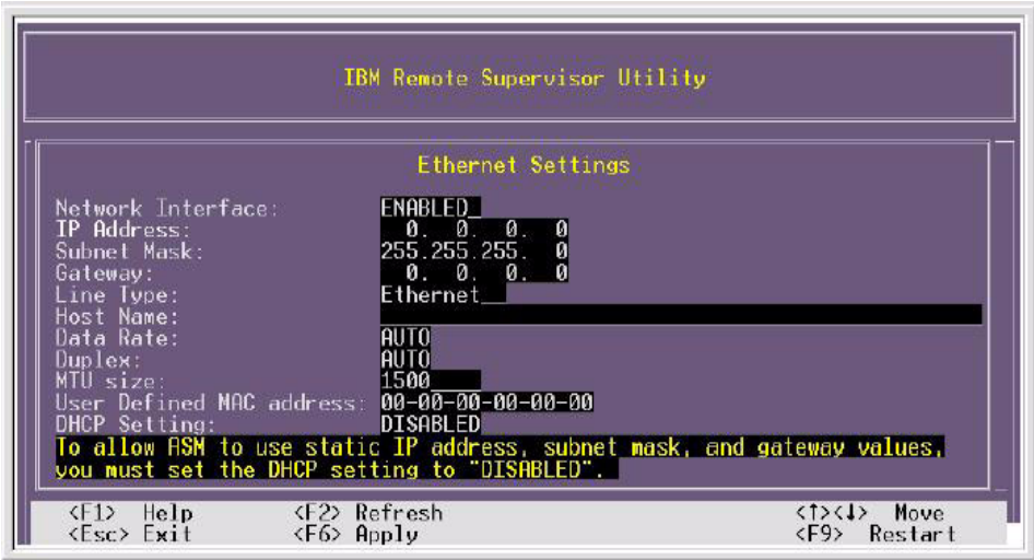
Figure 5-6 IBM Remote Supervisor Utility - Ethernet settings
