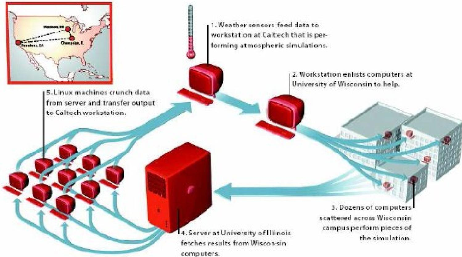
Figure 1.17 An example computational Grid built over specialized computers at three resource sites at Wisconsin, Caltech, and Illinois. (Courtesy of Michel Waldrop, "Grid Computing", *IEEE Computer Magazine*, 2000. [42])
