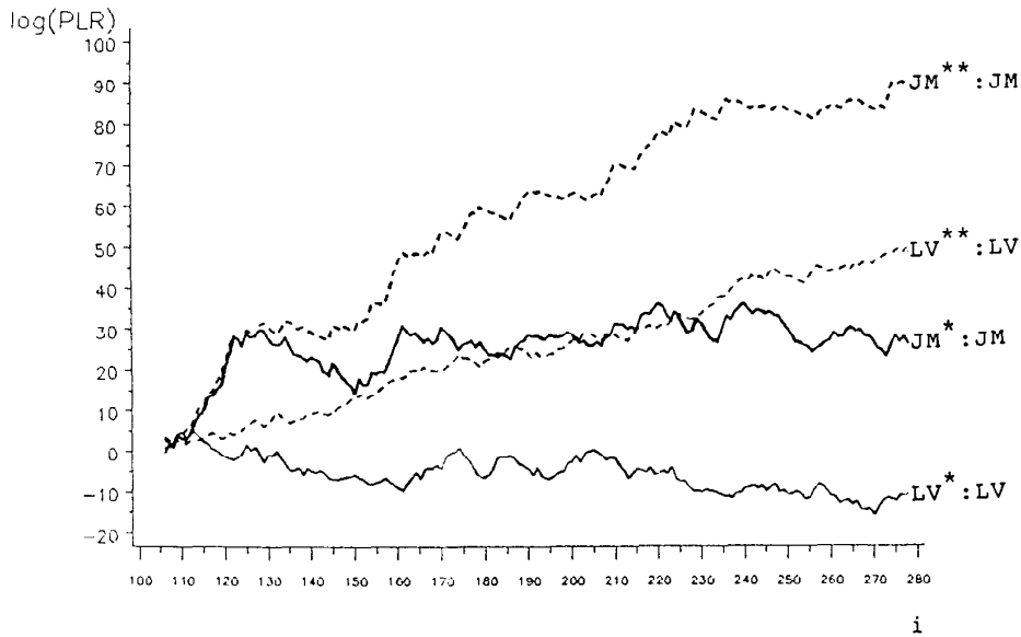
Fig. 10. Plot of log PLR against i , showing comparison of predictive accuracy between each type of recalibration and the raw predictions: JM and LV models, Musa SS3 data.
