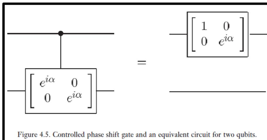
Figure 4.5. Controlled phase shift gate and an equivalent circuit for two qubits.
