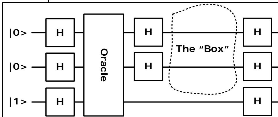
Verify that the gates in the dotted box in the figure perform the following conditional phase shift operation up to an unimportant global phase factor:
