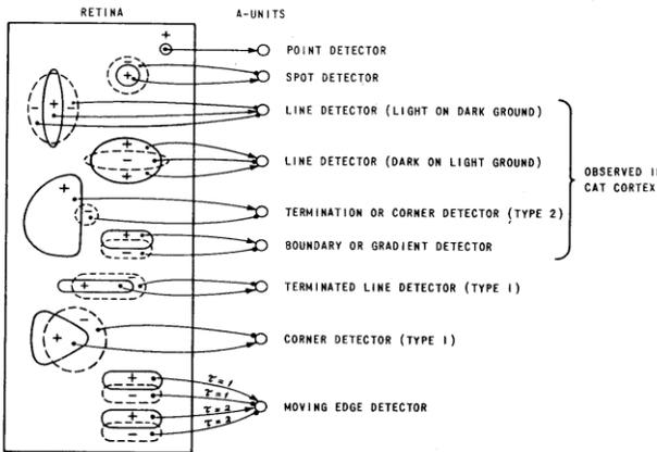
Fig. 10. Biologically plausible A1-units: broken lines indicate inhibitory fields, solid lines excitatory fields [13].
