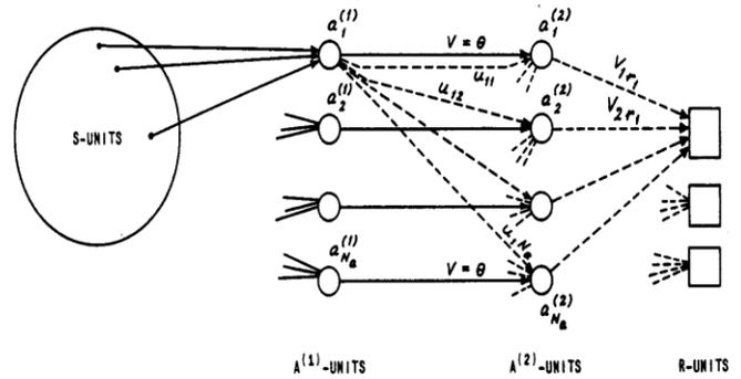
Fig. 12. Perceptron with two variable weight sets (dotted lines) [13].
